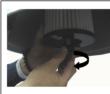
D. Unscrew and take out the HEPA filter
